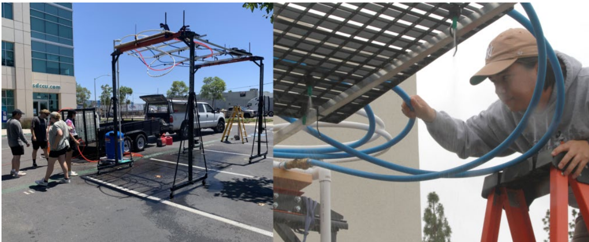
A field crew tests a custom-built rainfall generator that creates controlled rainfall patterns across 84 square feet of surface area. Right, Jerod Gray inspects the rainfall generator's nozzles. The field-deployable instrument is being used in an ongoing SMC effort to measure the effectiveness of routine street sweeping in preventing contaminants from entering storm drains and contributing to downstream water quality impairments.
