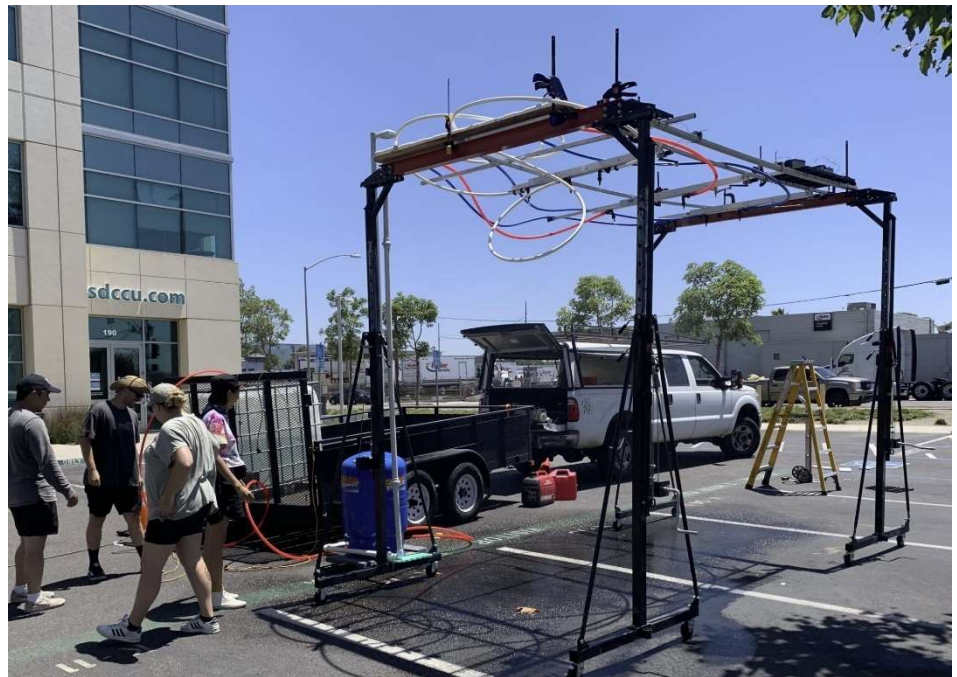
An SMC field crew tests a custom-built rainfall generator that creates controlled rainfall patterns across 84 square feet of surface area. The SMC is using the rainfall generator to investigate the effectiveness of routine street sweeping in removing contaminants that enter storm drains and contribute to contamination of downstream ecosystems.
