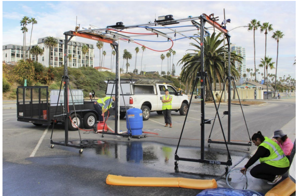
A field crew uses a custom-built rainfall generator to create controlled wet-weather conditions in a Long Beach parking lot – part of an SMC project to quantify street sweeping’s effectiveness in preventing roadway pollution from entering storm drains. Street sweeping is considered a type of non-structural BMP. Results are expected in 2025.
