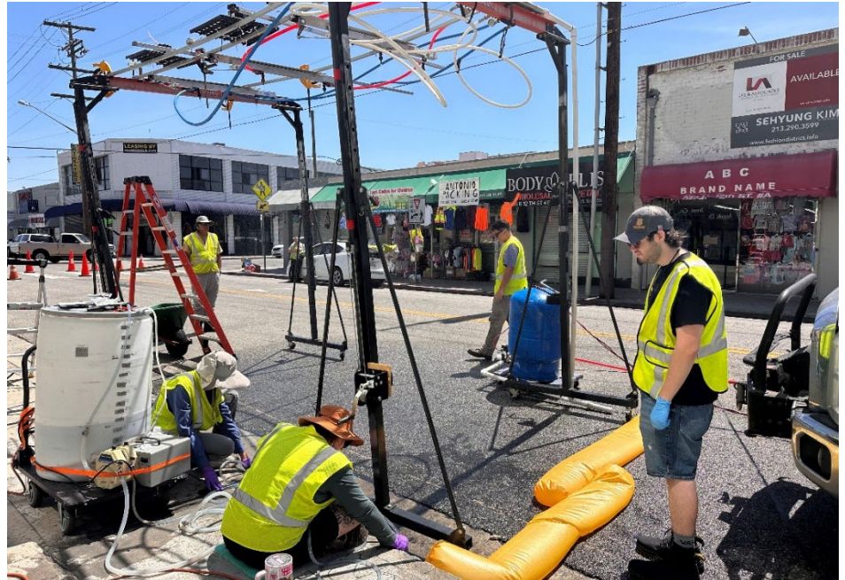
An SMC field crew sets up a custom-built rainfall generator on a commercial street in Los Angeles to create controlled wet-weather events, part of an ongoing study to measure the efficiency of routine street sweeping in removing pollutants that would otherwise enter storm drains and contribute to runoff pollution. Street sweeping is a common type of non-structural BMP.
