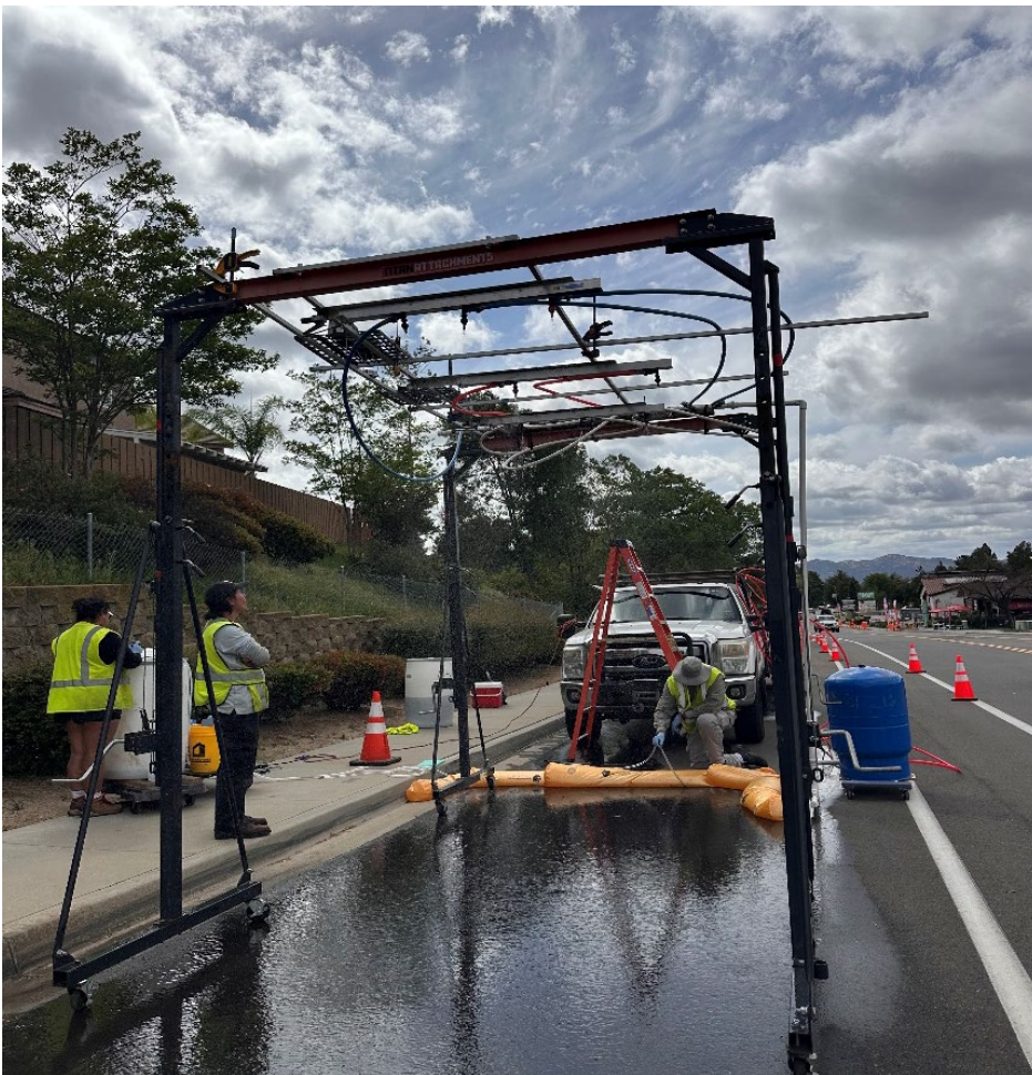
An SMC field crew collects runoff generated by a custom-built rainfall generator in a residential neighborhood in San Diego. Researchers are working to determine if runoff water quality is improved at segments of roadway that are intentionally swept vs. not swept during routine street sweeping.
